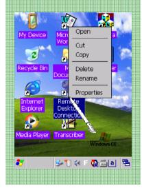
• **To drag** Similar function as mouse drag function of computer, with pressing screen, drag item to move to other position.
