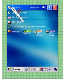
• Long Press After tapping, leave Stylus pen touching the screen. This function is frequently used for file copy, delete, and paste or with when keyboard is using.
